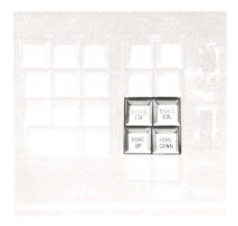
Unless the coded cursor key option is incorporated in a particular terminal, the cursor controls will not transmit a character and cause no action other than local cursor movement. (See Optional Features, page 8).
